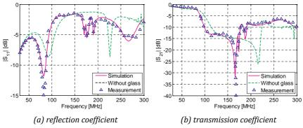
Fig. 12. Comparison of the measurement and simulation results for complex grid antenna
