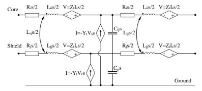
Fig. 39. Equivalent circuit for coaxial cable
