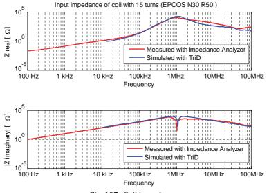
Fig. 107. Coil impedance
