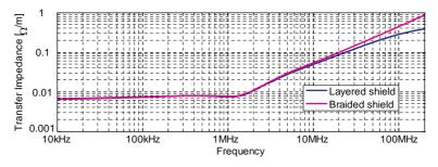
Fig. 71. Transfer impedance of braided and layered shields
