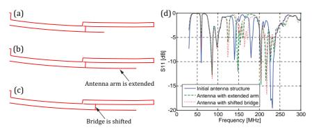
Fig. 27. Different variants of antenna structure: (a) initial structure, 102 metallic elements, (b) structure with extended arm, 117 metallic elements, (c) structure with shifted bridge, 117 metallic elements, and (d) reflection coefficient of the above antennas as a function of frequency
