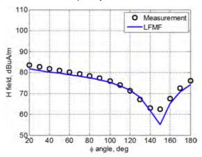
Fig. 97. H-field for the antenna located near the edge of the aluminium shield,  $\phi\text{-component}$
