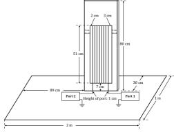
Fig. 10. View of the measurement setup for complex grid antenna
