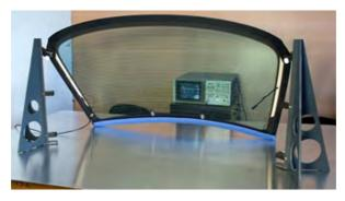
Fig. 13. Measurement setup for a rear-window automobile glass antenna
