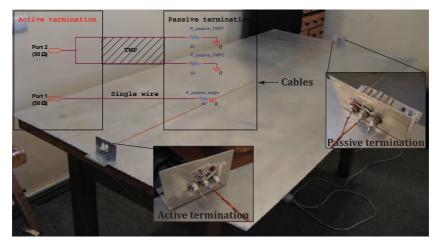
Fig. 42. Single wire and TWP cable. Measurement setup
