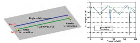
Fig. 43. Simulation model of a single wire and a TWP cable
