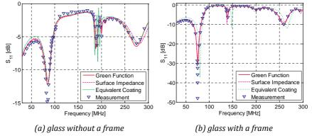
Fig. 9. Comparison between the simulation and measurement results
