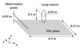
Fig. 84. A vertical loop above a finite plate
