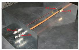
Fig. 63. Measurement setup: single cable and Coroplast 35 mm<sup>2</sup> cable with adapters
