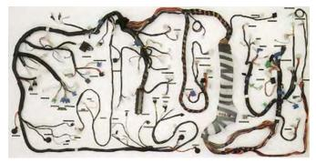
Fig. 36. Part of the cable harness of an automobile
