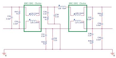
Fig. 108. Schematic of the filter under study
