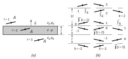
Fig. 6. Original (a) and equivalent (b) glass-antenna models
