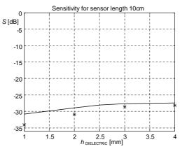
Fig. 61. Sensitivity vs. thickness of the dielectric substrate
