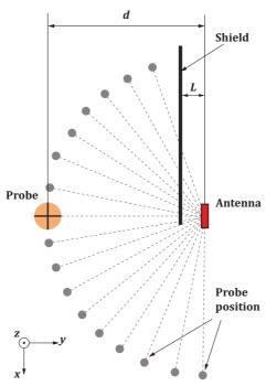
Fig. 95. A transmitting antenna with aluminium shield. Position of the shield: L=5 cm from the antenna centre. Position of the field probe: d=95 cm from the antenna centre
