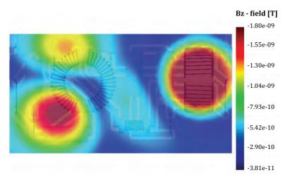
Fig. 117. Simulated vertical component of the B-field at 1 MHz for filter Model 1
