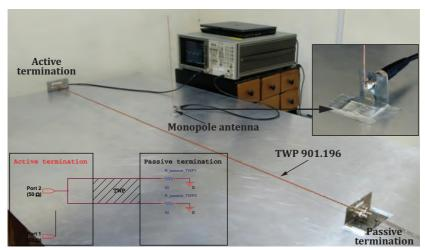
Fig. 45. Monopole and TWP cable. Measurement setup
