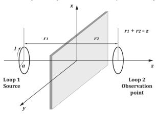
Fig. 82. Coaxial loops separated by an infinite plane [122]
