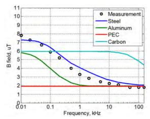
Fig. 88. Comparison of measured and calculated B-field in a car
