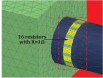
Fig. 74. Model for MoM calculations with solid shield and 16 SMD resistors
