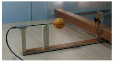
Fig. 91. Measurement setup with antenna in free space
