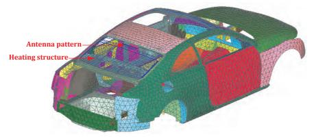
Fig. 26. Audi A5 car body with heating structure printed on the rear windscreen
