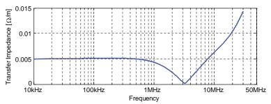
Fig. 79. Transfer impedance of layered shield of the Coroplast  $25 \text{\_mm}^2$  cable
