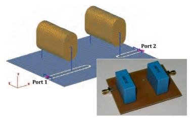
Fig. 103. Modelling of film capacitor
