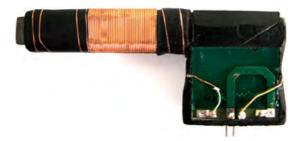
Fig. 90. Coil antenna of a smart-key system
