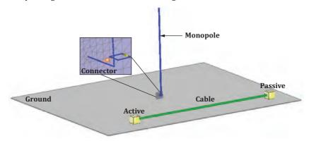
Fig. 46. Monopole and TWP cable. Simulation model
