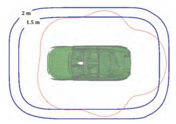
Fig. 99. Isoline representation of the B-field at 1 nT
