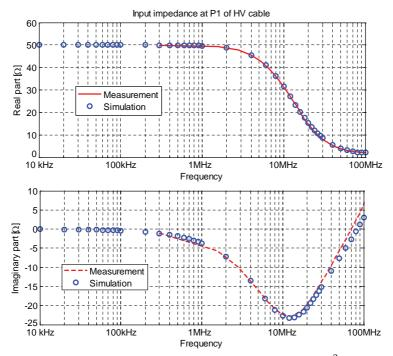
Fig. 80. Input impedance at Port1 of Coroplast 25<sub>mm</sub><sup>2</sup>
