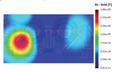
Fig. 116. Simulated vertical component of the B-field at 1 MHz for filter Model 2
