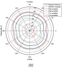
Fig. 33. Voltage received by antenna with different amplifiers as a function of azimuth angle of plane wave at a frequency 174 MHz: (a) vertical polarisation, (b) horizontal polarisation
