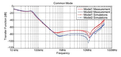
Fig. 112. Simulated and measured CM transfer functions
