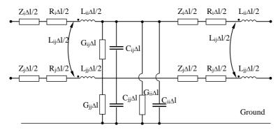
Fig. 38. Equivalent lumped-circuit model for two wires
