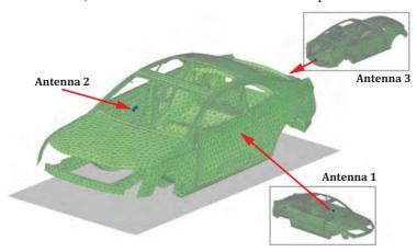
Fig. 98. Positions of three ferrite-rod antennas inside a car model
