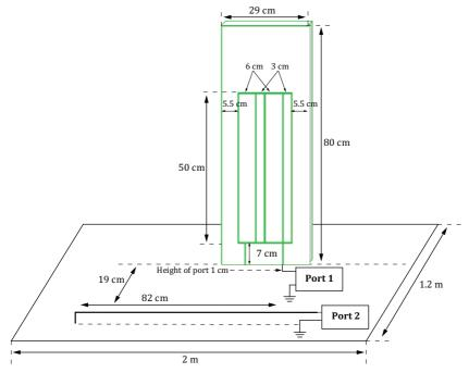
Fig. 50. Glass antenna and TWP cable. Setup schematic
