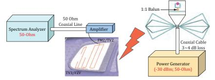
Fig. 18. Schematic representation of an antenna validation test
