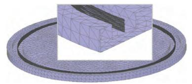
Fig. 101. Model details of the transmitting coil of an inductive charging system
