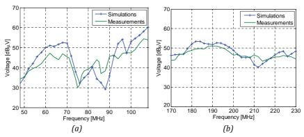
Fig. 24. Voltage received by TV2 antenna in (a) Band I and II, and (b) Band III
