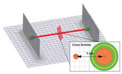
Fig. 65. Computational model for crosstalk analysis using an LCTL scheme of the transmission line
