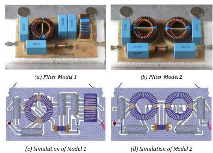
Fig. 109. Filter layouts and corresponding 3D models
