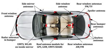
Fig. 4. Typical locations for antenna systems
