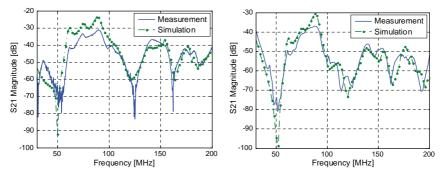
Fig. 54. Transmission coefficient (common mode)
