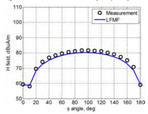
Fig. 94. H-field for antenna in free space, φ-component
