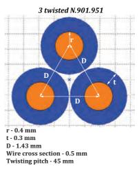
Fig. 41. 3-twisted wire cable
