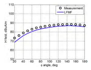
Fig. 96. H-field for the antenna located near the edge of the aluminium shield,  $\rho\text{-component}$
