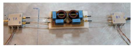
Fig. 110. Measurement of the DM transfer function
