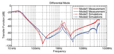
Fig. 113. Simulated and measured DM transfer functions
