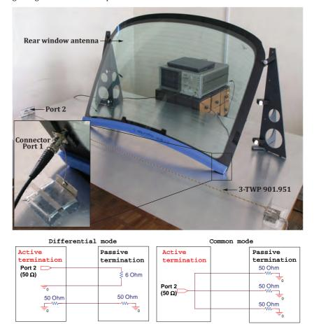
Fig. 53. Cable and car rear-window antenna. Measurement setup and schematic of cable terminations
