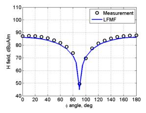
Fig. 93. H-field for antenna in free space, ρ-component
