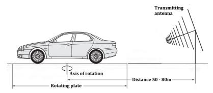
Fig. 28. Test setup for antenna pattern measurements
