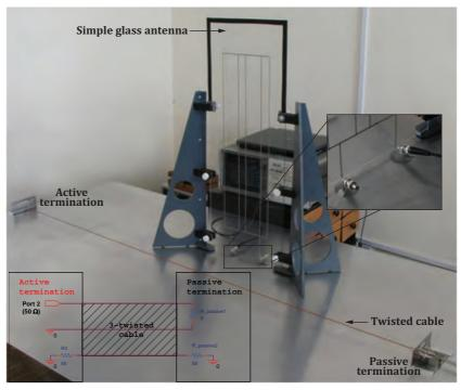
Fig. 49. Glass antenna and TWP cable. Measurement setup
