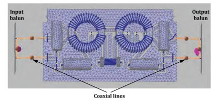
Fig. 111. Simulation model with baluns and coaxial lines
