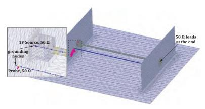
Fig. 75. Model for 3D simulations using MoM
