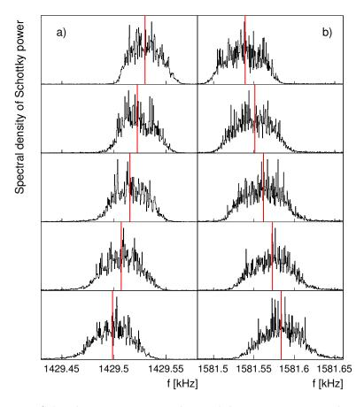
FIGURE 5.3: Schottky power spectra obtained during one 300 s cycle and scaled to harmonic number 1 for 1.0 GeV (a) and 2.0 GeV (b). The mean frequincies are indicated by the vertical (red) lines.
