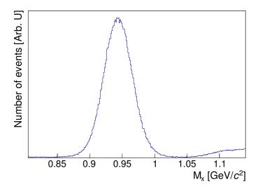
FIGURE 4.4: Missing mass  $M_X(pp \to pX)$  spectrum obtained from the particles detected in forward detector at the beam kinetic energy of 1.6 GeV.
