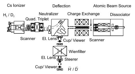
FIGURE 3.2: Set-up of the polarised ion source at COSY.
