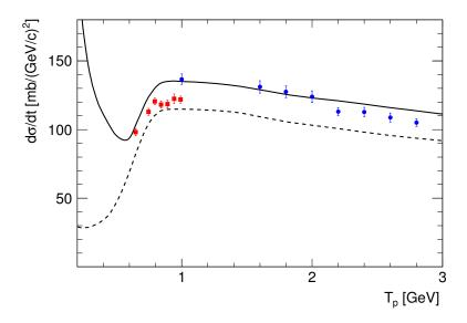
FIGURE 5.12: The predictions of Grein and Kroll [40] for the values of the forward pp elastic differential cross section (solid line), the corresponding lower limit provided by the spin-independent optical theorem of (Equation 5.13) being indicated by the broken line. The extrapolated ANKE data, corresponding to the A(Corr.) parameter of Table 5.2, are shown with their quoted errors by the (blue) circles, whereas the (red) squares are the published IKAR values [35].
