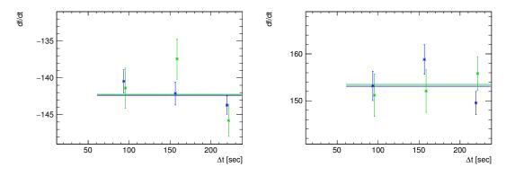
FIGURE 5.5: Average frequency shifts within the cycle duration, measured by new (blue) and old (green) spectrum analysers at 1.0 and 2.0 GeV.
