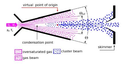
FIGURE 3.6: Cluster production at the Laval-nozzle.
