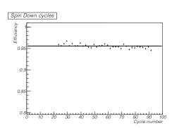
FIGURE 4.10: Efficiency of the elastic event reconstruction in FD in the cycles with the beam polarisation mode up (left panel) and beam polarisation mode down (right panel).
