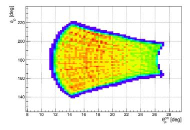
FIGURE 4.5: Forward detector angular acceptance for  $pp \to pp$  at the beam kinetic energy of 1.6 GeV.
