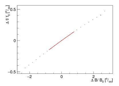
FIGURE 5.7: Variation of the mean revolution frequency with the field strength in the bending magnets for  $2.0~{\rm GeV}$
