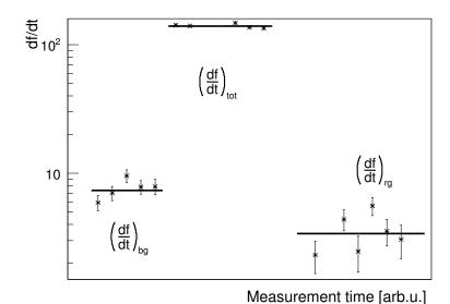
FIGURE 5.6: Example of frequency shift caused by the background when the target is on  $\left(\frac{df}{dt}\right)_{bg}$  (left) and when the target is off  $\left(\frac{df}{dt}\right)_{rg}$  (right) compared to the total frequency shift  $\left(\frac{df}{dt}\right)_{tot}$  with the beam incident on the target (middle).
