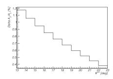
FIGURE 4.8: Systematic error due to the shift of the scattering angle. Example plots are shown for the beam kinetic energies  $T_p = 0.796$  GeV (left panel) and 2.368 GeV (right panel).
