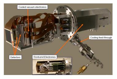
FIGURE 3.7: Silicon Tracking Telescope.
