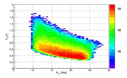
FIGURE 6.7: The ANKE acceptance in terms of the  $P_{sp}/P_t$  ratio dependence on c.m. the scattering angle at the beam energy pf  $T_p = 796$  GeV.
