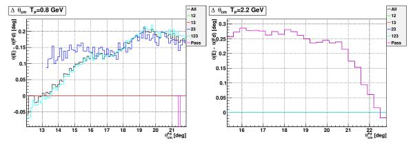
FIGURE 4.7: Difference of scattering angle reconstructed in FD and STT. Example plots are shown for  $T_p=0.796$  GeV (left panel) and 2.157 GeV (right panel).
