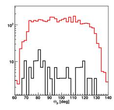
FIGURE 6.1: The acceptance  $pd \to ppn_{sp}$  (black histograms) and  $pd \to pnp_{sp}$  (red histograms) reactions simulated in the framework of spectator model at  $T_p$  = 0.796 GeV. One proton is detected in the FD and other one in the STT1 (left panel) or in the STT2 (right panel).
