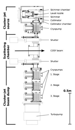
FIGURE 3.5: The cluster-jet target installed at ANKE.
