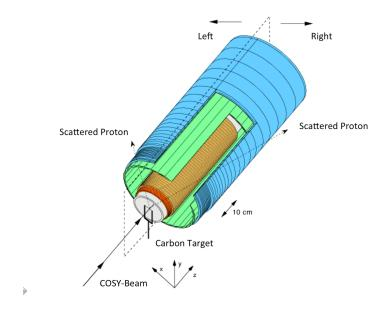
FIGURE 3.3: Schematic diagram of the EDDA detector.
